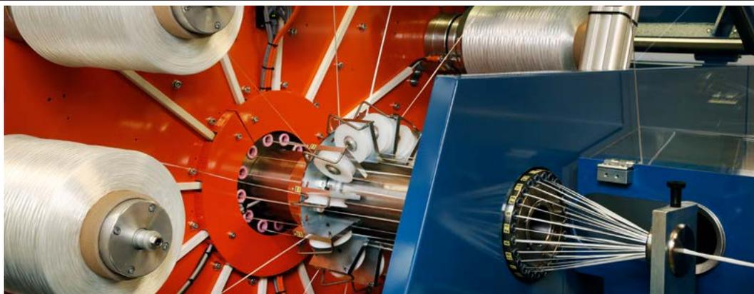
Roblon servers utilise a unique tension system, where yarns are controlled individually and precisely by a combination of hysteresis brakes and state of the art control software.
